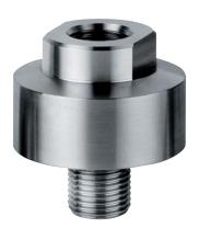
Diaphragm seals are designed to isolate the sensing element of pressure gauges and pressure switches from process fluids that may be corrosive, viscous, sedimentous and/or with a high temperature. The diaphragm is welded to the body, to ensure separation of the filling fluid from the process medium. The threaded connection make it easy to use on all applications where the reduced size of the system is important and also where gauges of 2.5" (63 mm) diameter are required.
